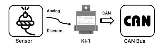
The Ki-1 is an ideal solution for converting signals from one or two sensors with current, analog or digital outputs into a digital CAN signal when installing an electronic unit with more inputs is not practical.
