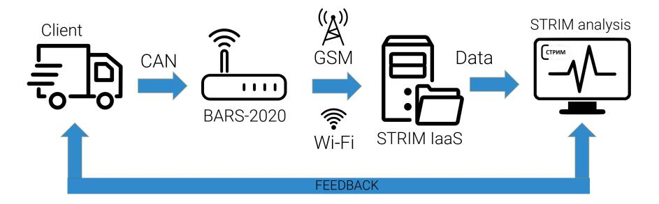
The data coming from the BARS-2020 recorder to the STRIM server is processed and analyzed by our specialists. The result of this analysis is the feedback with the Client, allowing you to improve the efficiency and safety of machine operation.
