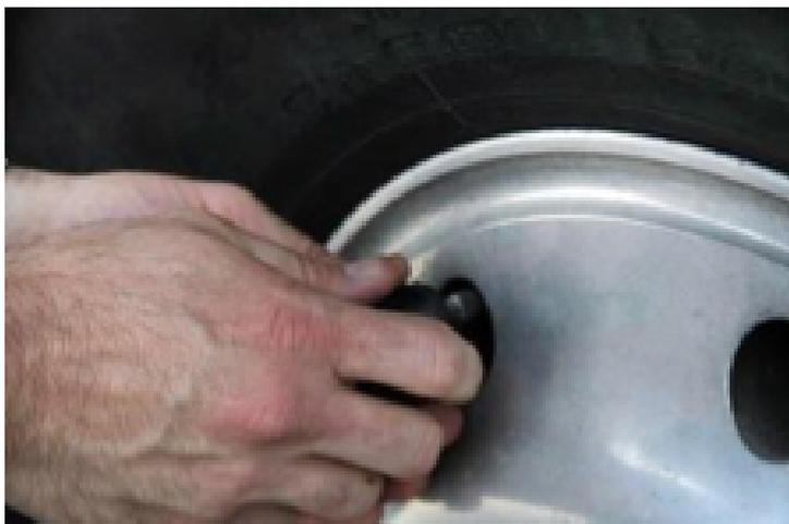
Figure 44: Installing the sensor on the tire valve
