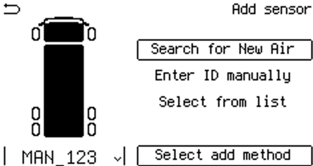
Figure 42: Sensor adding methods
